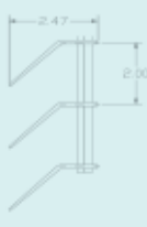
VisiShield LG-75 Open Area: 64% Visual Block: 75%
