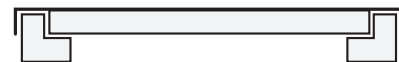
Style F: Deck with waterfall end plate on top of on step beam
